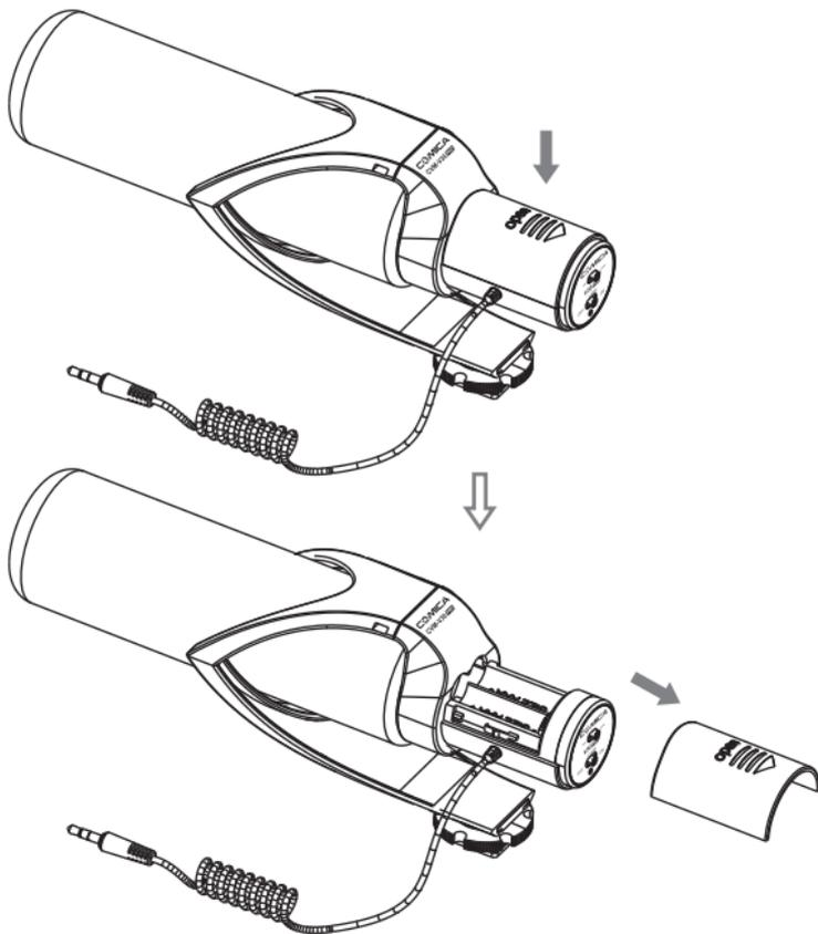
1.12 Put into the batteries, and then push forward to close the battery door
