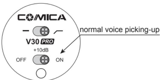
2.32 Switch the button to '+10 dB' position, then the sensitivity can be increased with 10 dB, The recording sound will be increased accordingly
